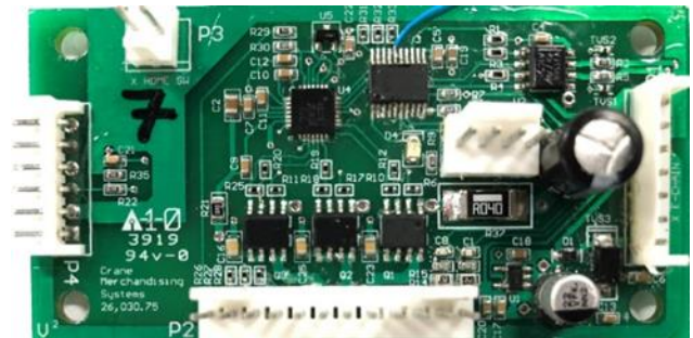
Cabinet X Motor Control Board
